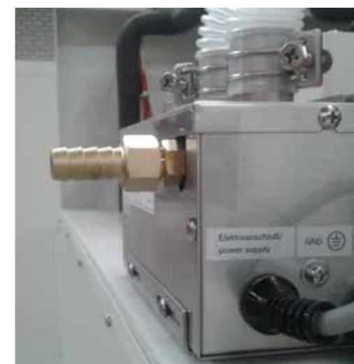
Water inlet for the Ultrasonic humidifier.
